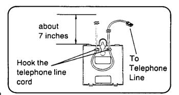
4 Insert the hook of the wall-mounting adaptor into the hole of the unit then place the wall-mounting adaptor by pushing it in the direction of the arrow **A**, as shown.
